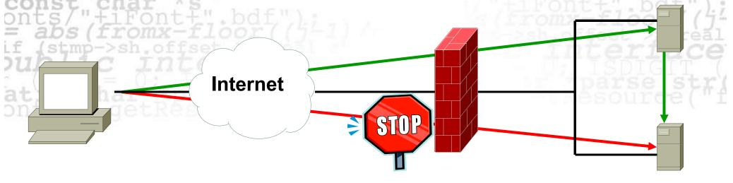
Use alive6-remote for checking if routing headers are allowed to target
