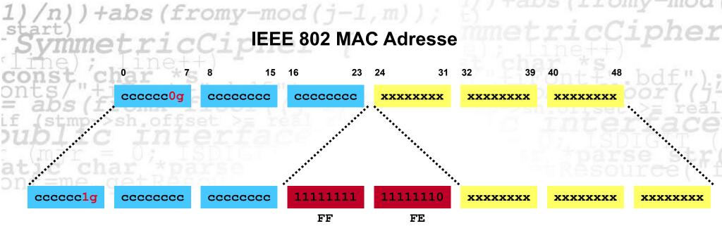
IPv6 Interface Identifier im EUI-64 Format EUI: Extended Unique Identifier
